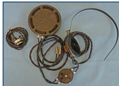
Notice the clip on ear piece that went just over one ear. Batteries and microphones were hidden on various parts of the body. All body aids from this era had problems with clothing rubbing over the microphone causing a tactile vibration that sounded like static.
