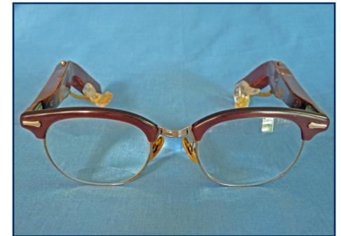
Here is a Sonotone transistor eyeglass hearing aid from the 1950's. These were a revolutionary improvement over vacuum tube aids. Smaller, more convenient and more durable, these were very popular. Still, they had only three to six transistors and basically were amplifiers that amplified too much background noise.
