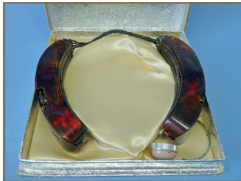
The Acousticon A-200 (Barrette) hearing aid required both barrettes to contain all the electronic components and batteries.
